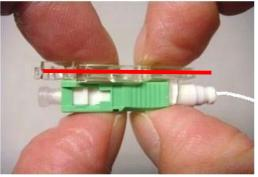
② Re-attach the clear wedge onto the connector. Ensure that there is no space between the wedge and the connector.
